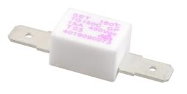
DC Alloy Thermal-Link is defined as a non-resettable protective device functioning one time only. It is widely used in electrical equipment and electric vehicle. Normally, thermal element is jointed to the two electrode leads. Under abnormal conditions, when the temp. reaches to the fusing temp. of Thermal-Link, the thermal element melts to disconnect the circuit completely and quickly retracts to the two electrode lead ends with the aid of the flux.
