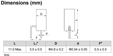
a: F,  $L_1$  and the bending mode of pins can be customized as required.
